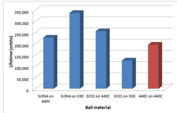
Figure 6. Normalised lifetimes of MoS<sub>2</sub> lubricated ceramic balls, in comparison to steel-on-steel [1]
