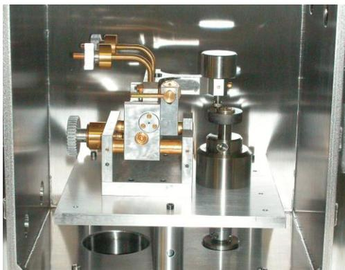
Figure 1. Vacuum pin-on-disc tribometer
