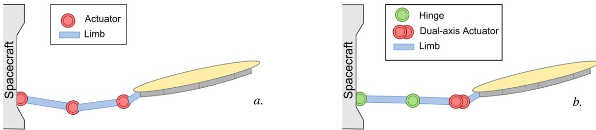
Figure 2. Reflector boom concepts with rotary actuators at the joints (a.) and single rotation hinges (b.). (Rotation axes not shown.)
