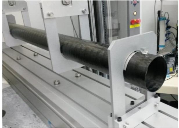
Figure 6. CFRP Tube in four-point bending test set-up.
