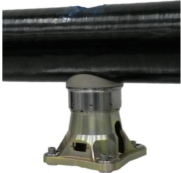
Figure 9. NELS Hold-down and release mechanism adapted for the reflector boom.
