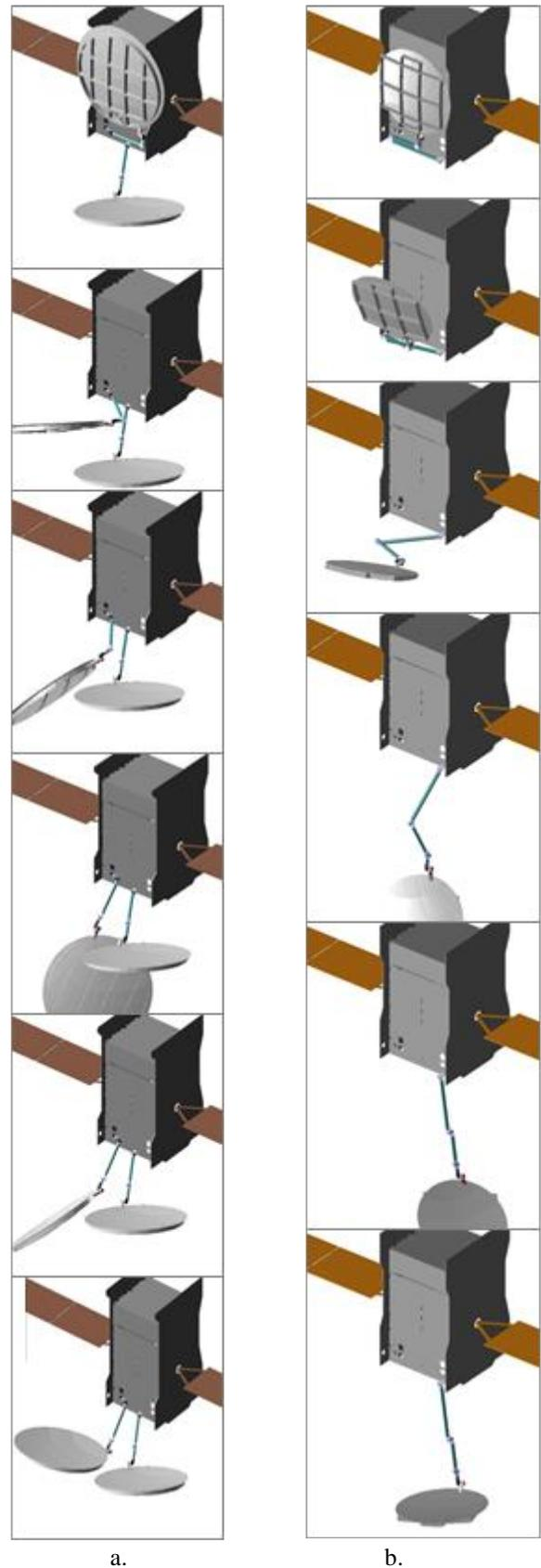
Figure 4. Deployment trajectories of two reflector boom variants: a.) two-hinge variant; b.) three-hinge variant.
