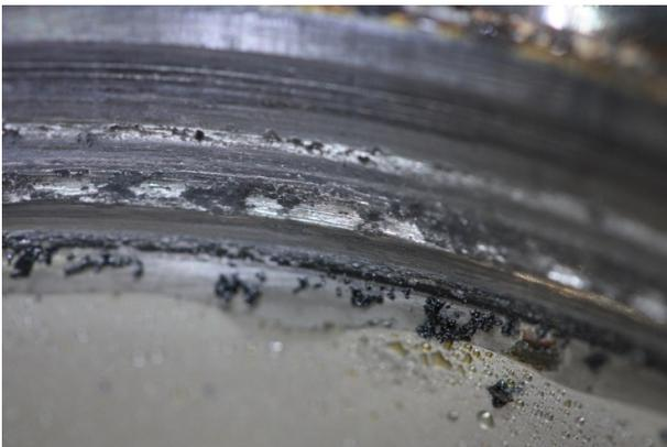
Figure 7. Showing wear on bore of flexspline
