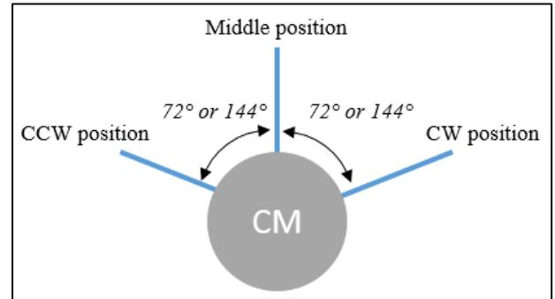
Figure 10: Angular repeatability test
