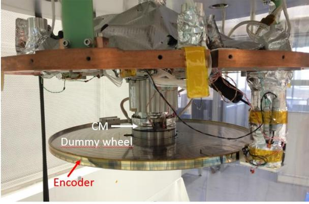
Figure 9: CM and its wheel installed in cryostat
