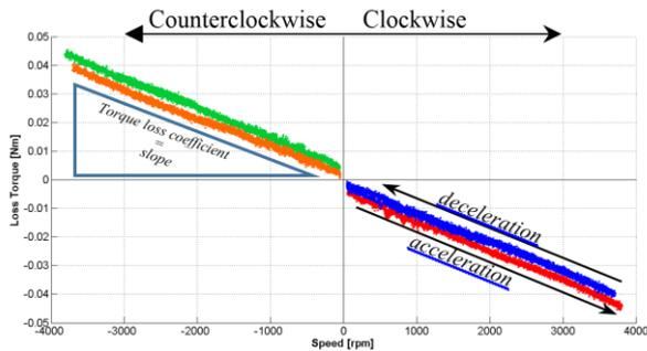
Figure 2-3 Results of the full speed full torque test
