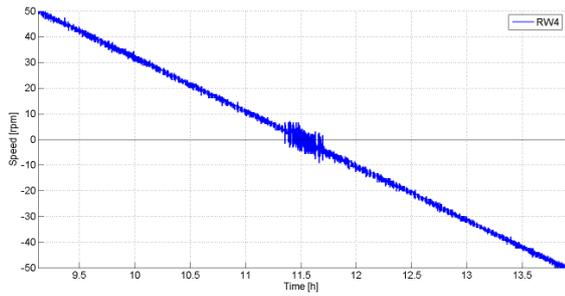
Figure 3-1 Wheel speed zero crossing on-orbit
