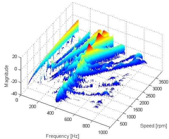
Figure 2-4 Integral flight spare RW waterfall plot
