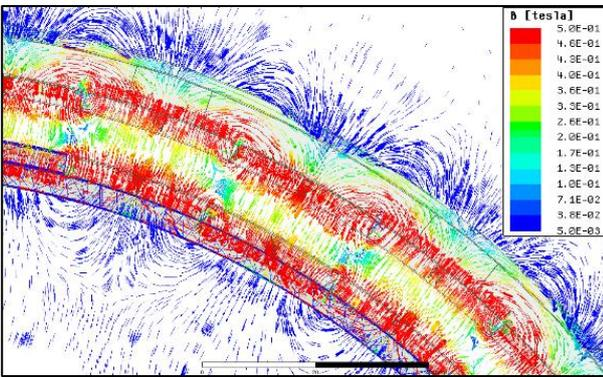
Figure 4-2: B-field vector plot of the motor airgap
