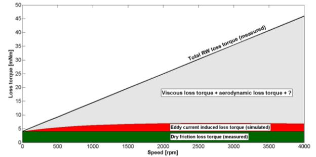
Figure 4-4: Assumed loss torque composition (for the Integral RW)
