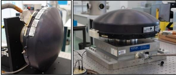
Figure 2-1: Integral flight spare reaction wheel on torque transducer (left) and on Kistler table (right)
