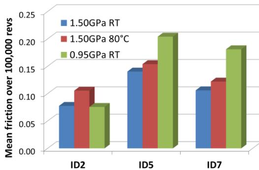
Figure 4. Mean friction over 100,000 revs of IL-lubricated PoD tests under vacuum
