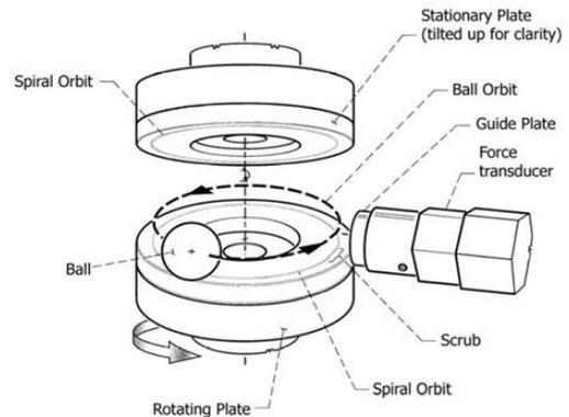
Figure 6. Internal arrangement of SOT
