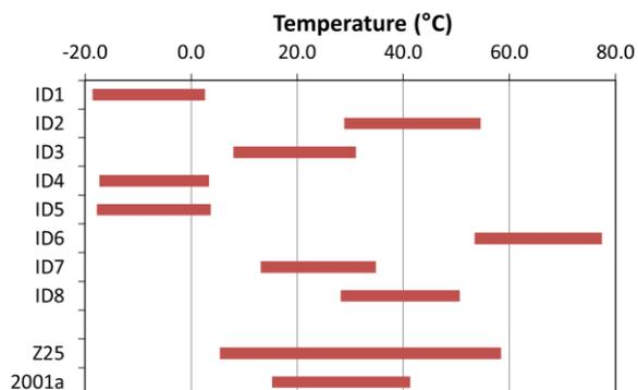
Figure 1. Temperature ranges at which ILs, Z25 and 2001a provide viscosities of 100-400 mm<sup>2</sup>/s
