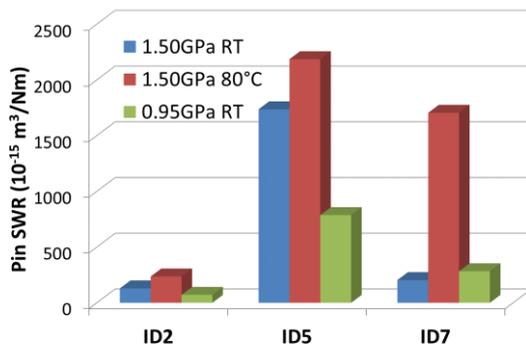
Figure 5. SWRs of test pins lubricated with ILs
