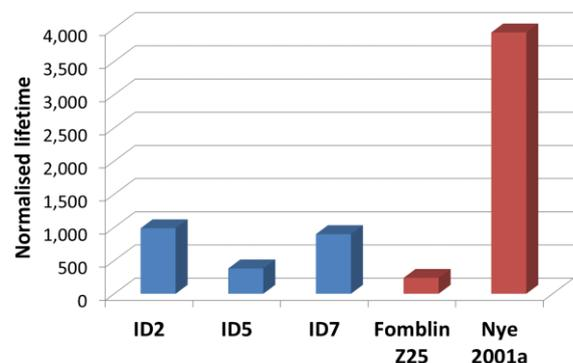
Figure 7. Rolling lifetimes of ILs under vacuum on the SOT
