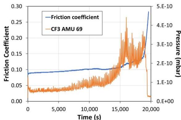
Figure 7.  $CF_3$  behaviour during ID2 test (2.25GPa, RT)
