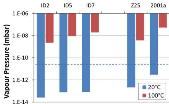
Figure 3. Vapour pressure measurements of down-selected ILs, Z25 and 2001a. Line indicates specification value @ 20°C
