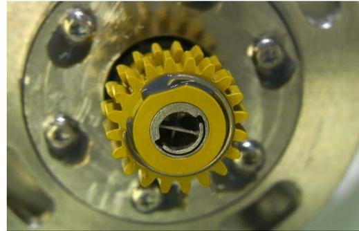
Figure 7. SADM high-speed potentiometer anti-backlash pinion system in Duratron.
