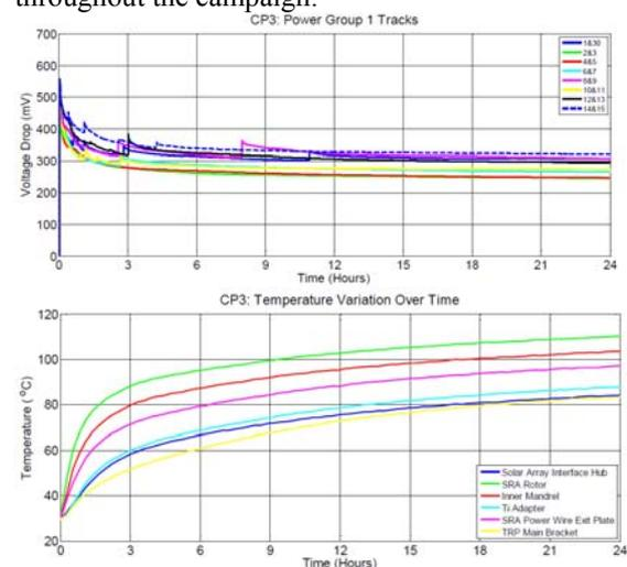
Figure 11. Voltage drop in slipping power tracks at 12.5A and the temperature increase during 24 hours
