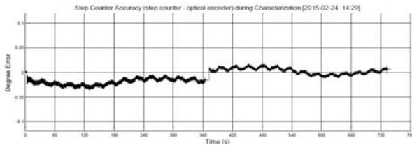
Figure 6. Accuracy between step commands and SADM shaft position measured by an external encoder for 360° step in both directions.
