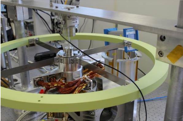
Figure 13.  $2.5 \text{ kgm}^2$  dummy inertia load and aluminium torque rod that yields in torsion simulating higher torque loads.
