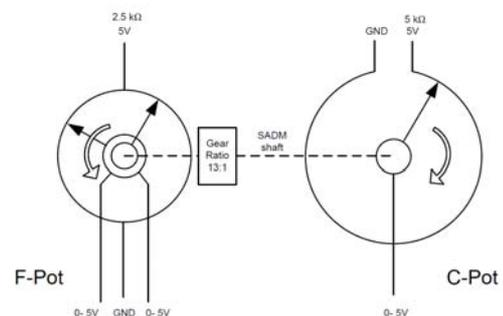
Figure 10. SADM high-speed and slow-speed potentiometer.
