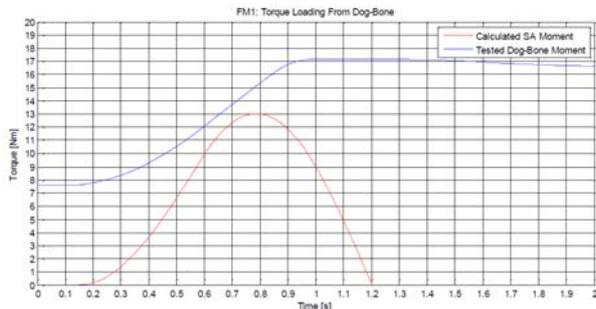
Figure 14. Moment in aluminium rod under acceleration of SADM to  $6^\circ/s$  with  $12^\circ/s^2$  overlapping calculated inertia loading from Solar Array.
