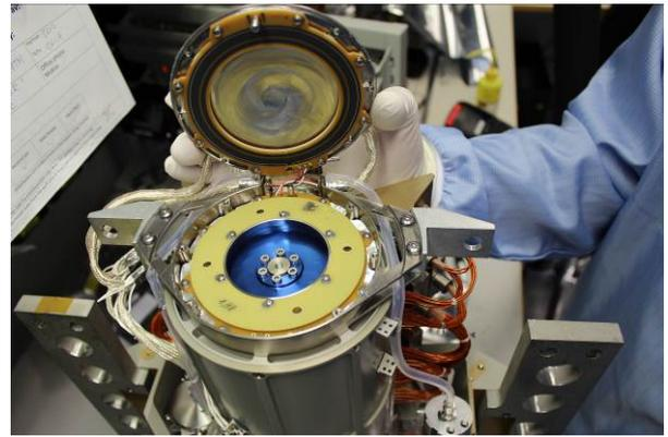
Figure 4. Slipring aft end with potentiometers and (blue anodized) titanium alloy diaphragm providing axial compliance for the ball bearing.
