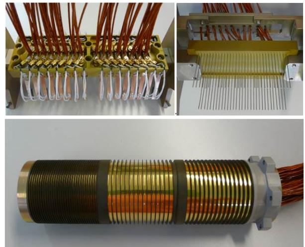
Figure 5. Slipring brush blocks and rotor using hybrid track technology for power and signal
