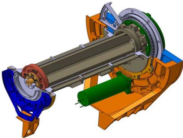
Figure 3. SADM mechanism structural build up
