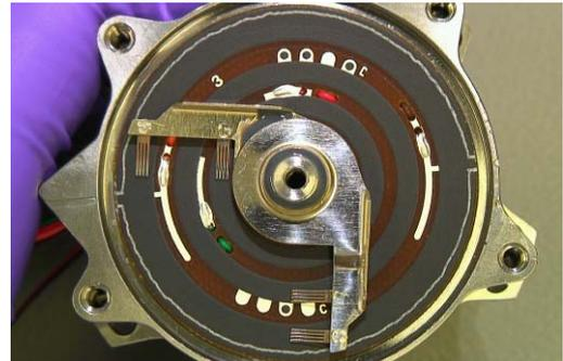
Figure 8. SADM high-speed potentiometer with dual wipers.
