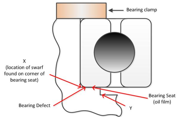
Figure 15. Bearing setup showing locations of findings
