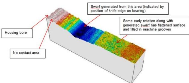
Figure 13. 40x amplification 3D profile of a slide of the bearing seat
