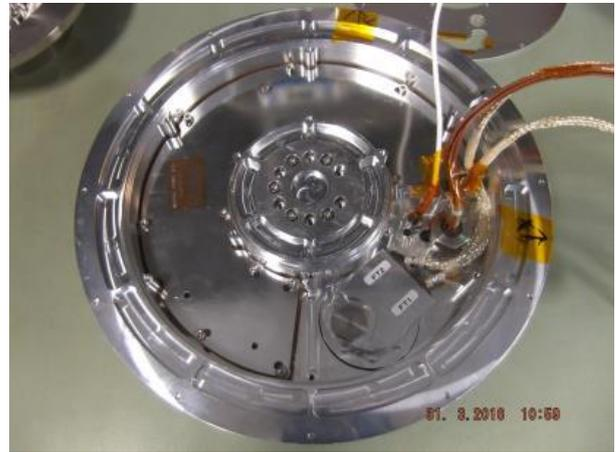
Figure 7. ACM ready for disassembly (mechanism still in vacuum)
