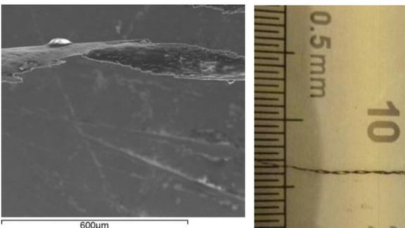
Figure 10. ACM upper bearing seat swarf found
