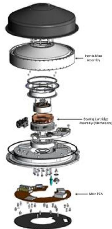
Figure 19. SSSL's First Generation Geo Wheel
