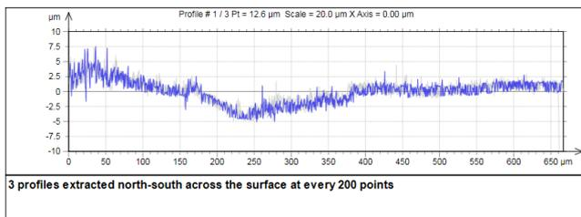
Figure 14. Approximate width of groove shown of 150µm
