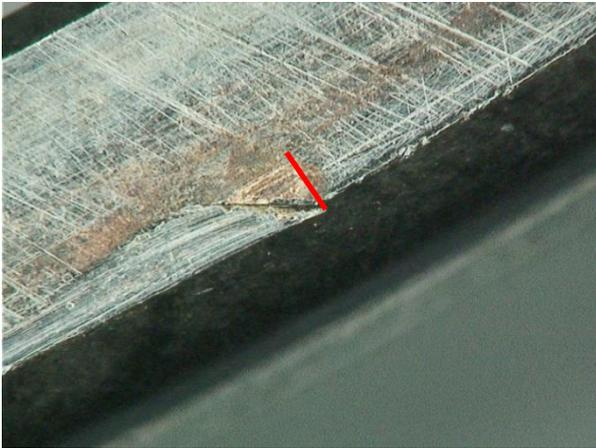
Figure 12. Bearing defect
