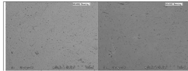
Figure 18. Micro-pitting of balls (SEM)
