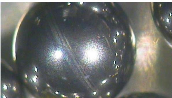
Figure 17. Ball with single orbital track
