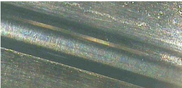
Figure 16. Bearing race showing running track
