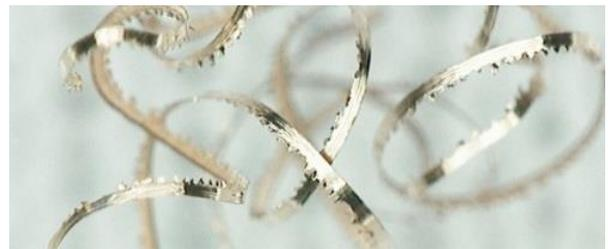
Figure 11. Swarf generated during machining operation
