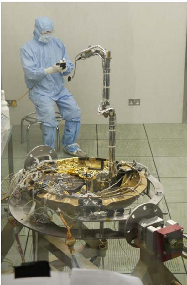
Figure 6: Instrument Arm Assembled in Lander
