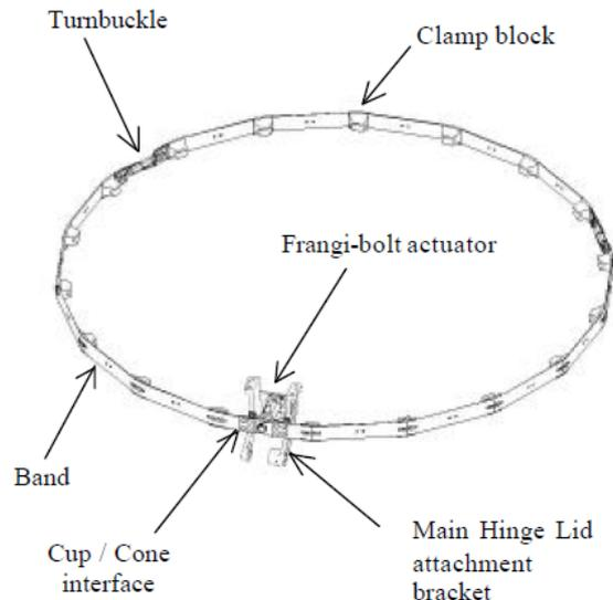
Figure 2: Clamp band Assembly (CBA)
