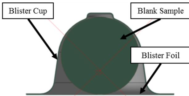
Figure 8. Section through Blister Package
