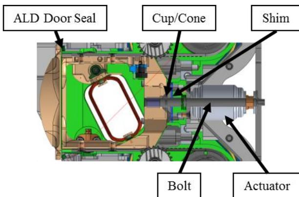
Figure 11. Section through the Release Bolt
