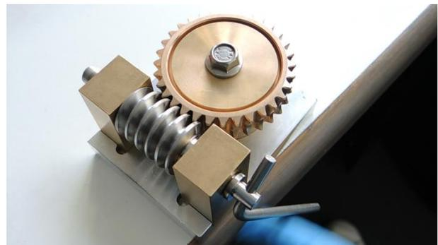
Figure 10. Example for jig to test gears
