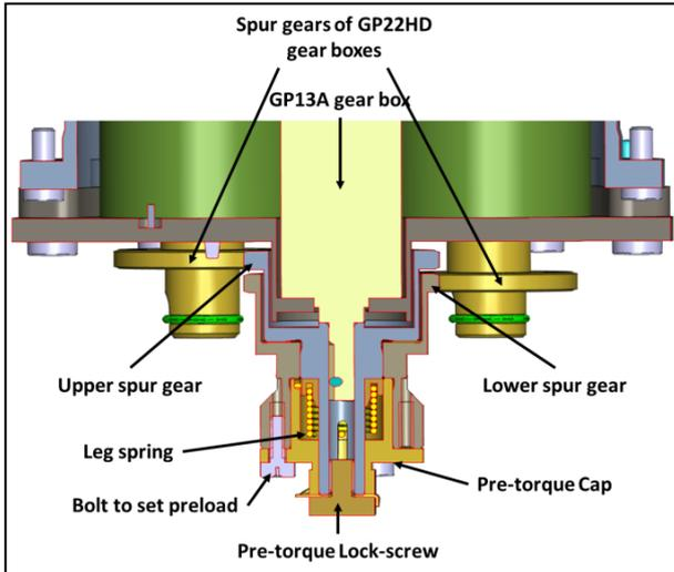
Figure 6. Pre-torque Device.
