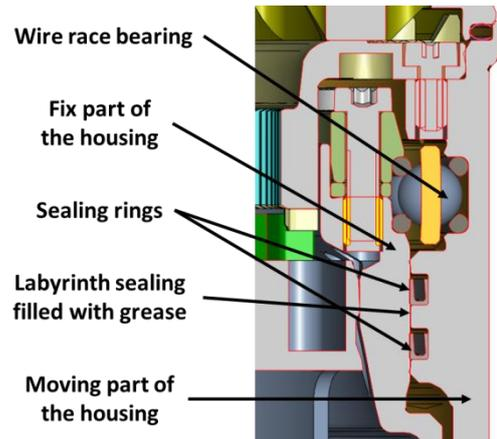
Figure 3. Design of "large" radial dynamic seal
