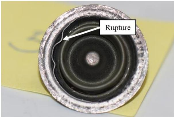
Figure 12. Ruptured Blister Cup
