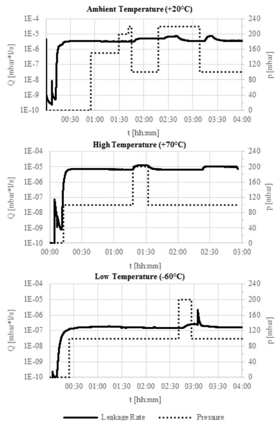
Figure 5. Leak plots for ambient, max. and min qualification temperature
