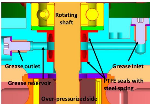
Figure 2. Design of "small" radial dynamic seal
