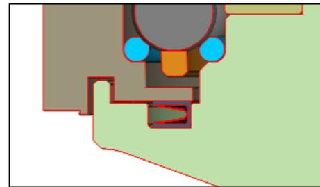
Figure 4. Design of axial dynamic seal
