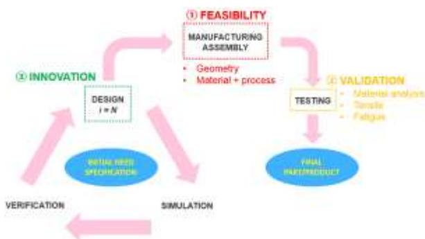
Figure 2. SLM compliant structures development steps
