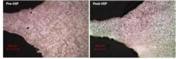
Figure 5. Sample cuts before and after HIPing.
