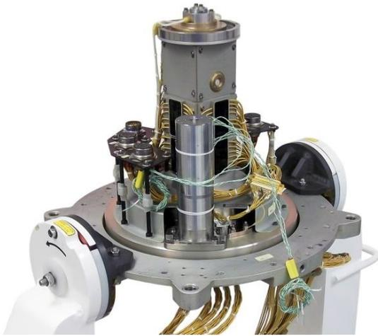
Figure 5. EuroSMG Breadboard on SADM
