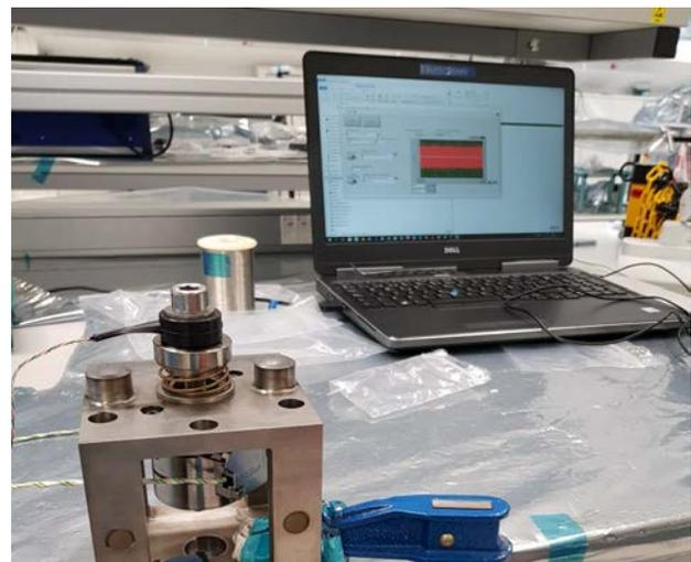
Figure 4. Preload characterization Test
