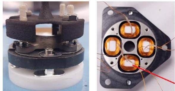
Figure 14: M-FSM45 tooling for mirror and moving part assembly (left) and coils potting (right)
