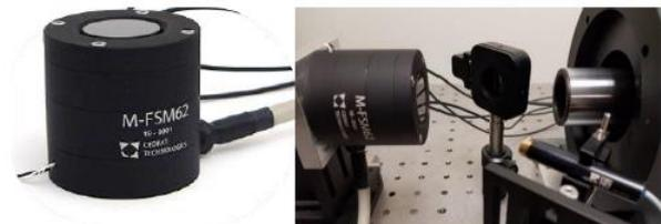
Figure 19: M-FSM62 on optical test bench
