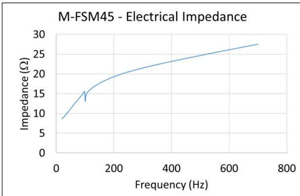
Figure 17: M-FSM45 Electrical impedance
