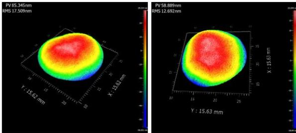
Figure 4: Mirrors RWE after integration M-FSM45 (left) P-FSM150S (right)
