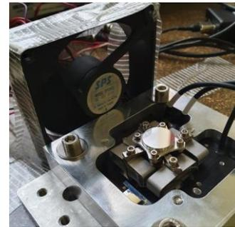
Figure 10: lifetime test set-up for PFSM150S EMI
