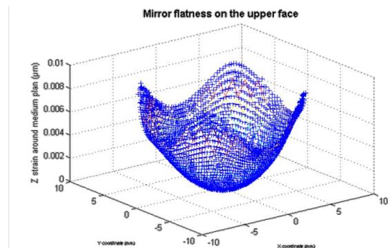
Figure 2: mirror deformation for a +60°C temperature
