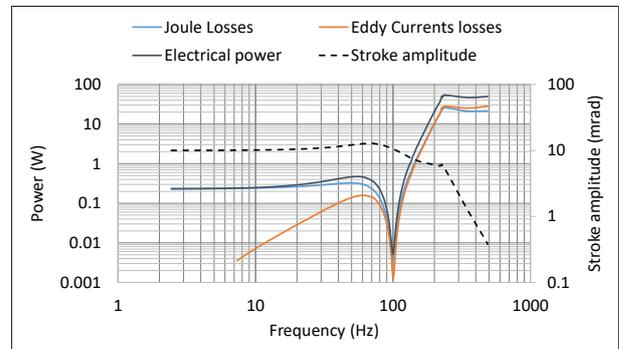
Figure 23: Power diagrams at +/-10mrad amplitude.
