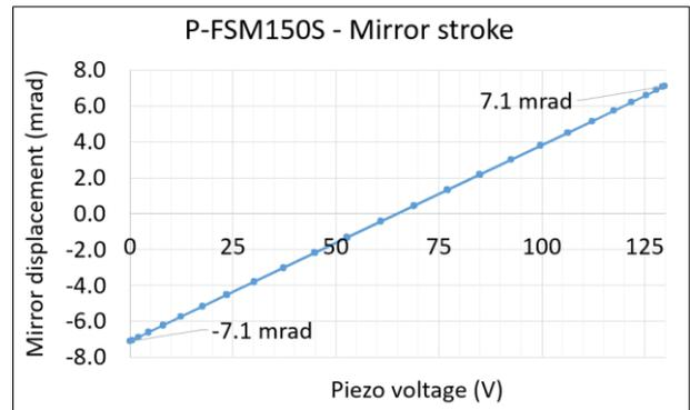
Figure 6: PFSM150S stroke results with a 0/+130V supply
