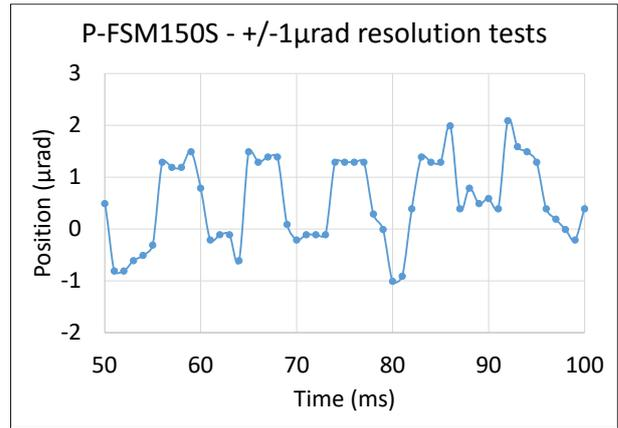
Figure 9: mechanical resolution test
