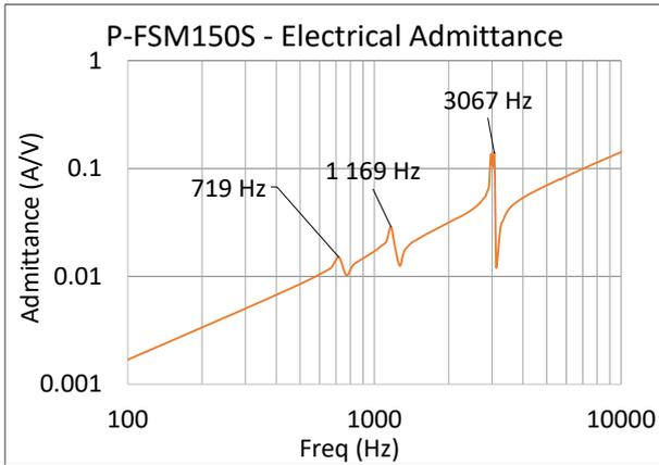
Figure 7: PFSM150S EMI X-axis admittance sweep
