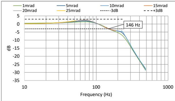
Figure 20: Bandwidth tests at different amplitudes.
