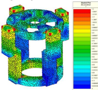
Figure 12: M-FSM Magnetic Finite Element Analysis
