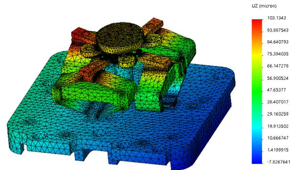
Figure 1: P-FSM150S simulation (vertical displacement) for a +60°C temperature
