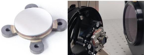
Figure 3: Free state mirror (left) and Mirrors RWE test after integration (right)
