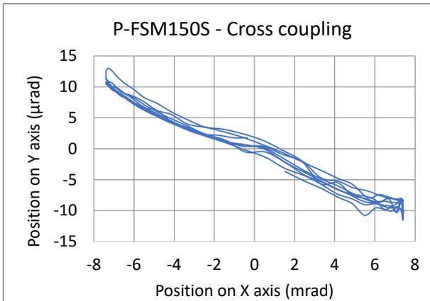
Figure 8: PFSM150S cross coupling measurement
