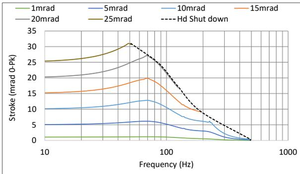
Figure 21: M-FSM62 Amplitude diagrams v.s electronics limits.
