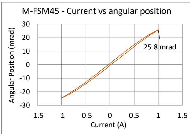
Figure 18: M-FSM45 stroke amplitude test
