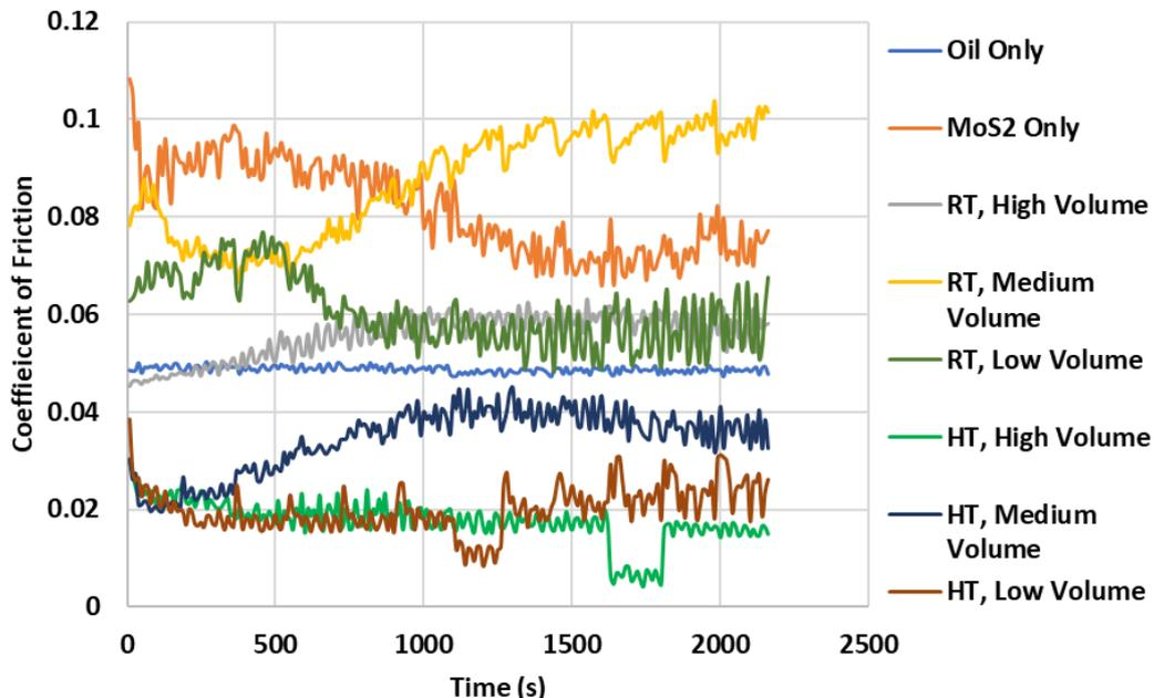
Figure 4 – Friction progression for MTM tests
