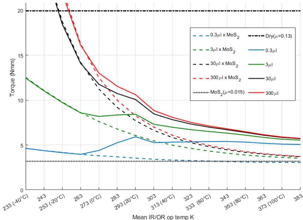
Figure 9 – Torque estimations for 7004C bearing pairs (31mm PCD) (iso-thermal housing), lubricated with Z25 only (solid) and hybrid lubrication (dashed), or varying volumes. “Dry” equates to no effective lubrication ( $\mu=0.13$ )
