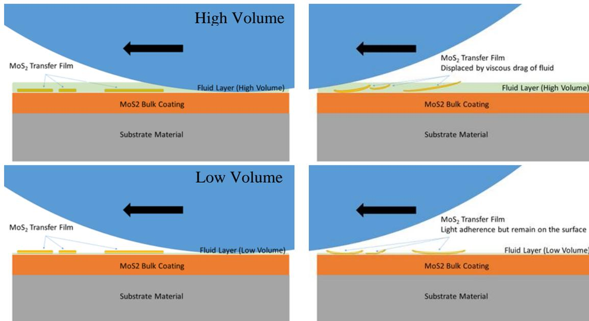
Figure 1 – MoS<sub>2</sub> transfer film formation (3<sup>rd</sup> body) for high and low fluid volume hybrid lubrication [2]
