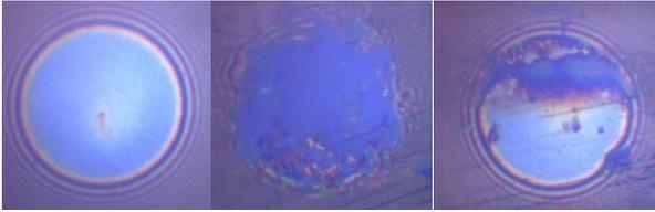
Figure 5 – Mid-test SLIM assessments for room temperature hybrid tests, with high fluid volume (left), medium fluid volume (centre) and low fluid volume (right)
