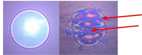
Figure 3 – End of test SLIM assessments for oil only (left) and MoS<sub>2</sub> only (right) MTM tests
