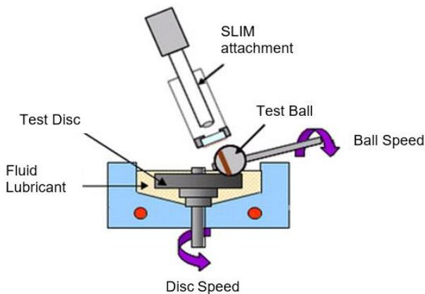
Figure 2 – Schematic of an MTM [5]
