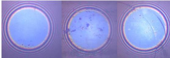
Figure 6 – Mid-test SLIM assessments for high temperature hybrid tests, with high fluid volume (left), medium fluid volume (centre) and low fluid volume (right)
