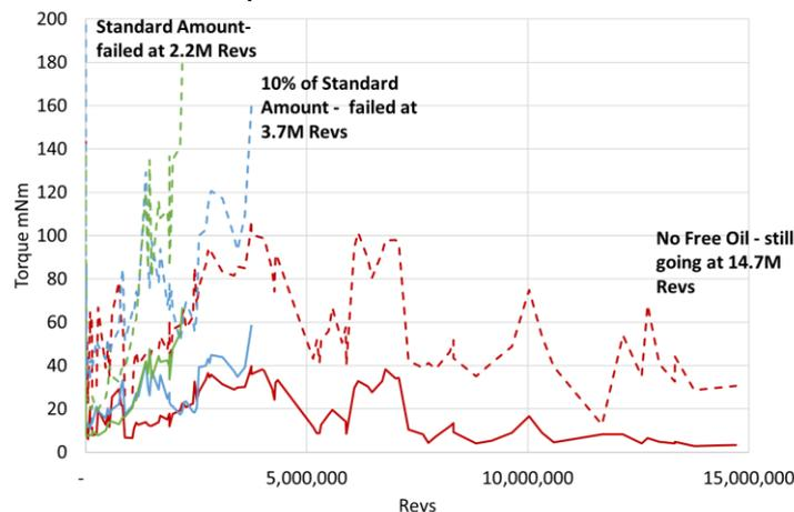
Figure 7 – Hybrid lubricated 7004C bearing lifetimes under vacuum (varying fluid volumes)
