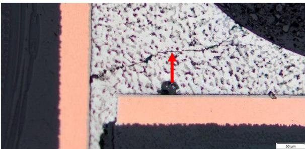
Figure 12. Micro section of the ground line solder joint: initial design
