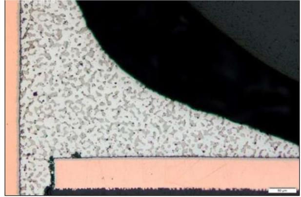
Figure 16. Micro section of the ground line solder joint: final design
