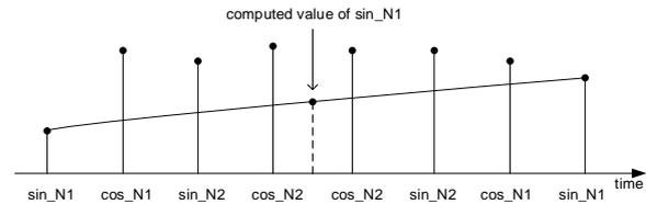
Figure 5. Acquisition schema of position sensor signals
