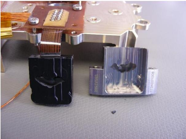
Figure 11. Read head failure due to thermal stresses
