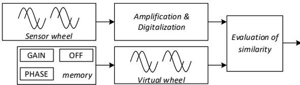
Figure 6. Concept of Novel Position Estimation Method
