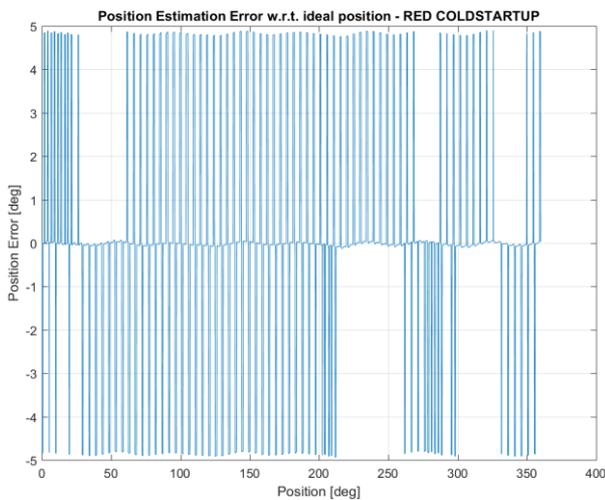
Figure 15. Position estimation reliability for FWS at cold start-up
