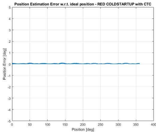
Figure 17. Position estimation reliability for FWS at cold start-up when using CTC
