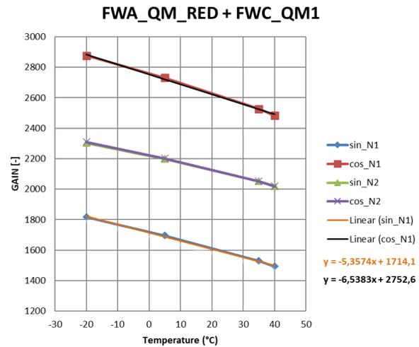
Figure 14. FWS gain thermal drift
