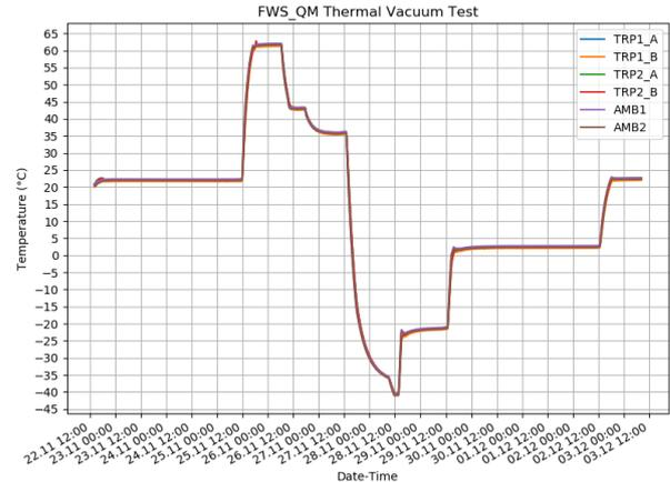
Figure 13. FWS first thermal cycle
