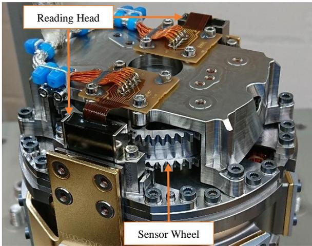
Figure 3. Filter Wheel Position Sensor
