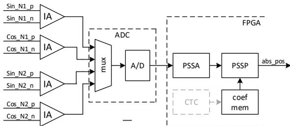
Figure 4. Scheme of Position Estimation Chain
