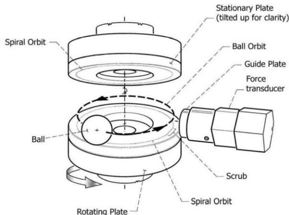
Figure 4. Internal arrangement of the SOT
