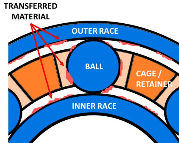
Figure 3. Double-transfer mechanism within a bearing
