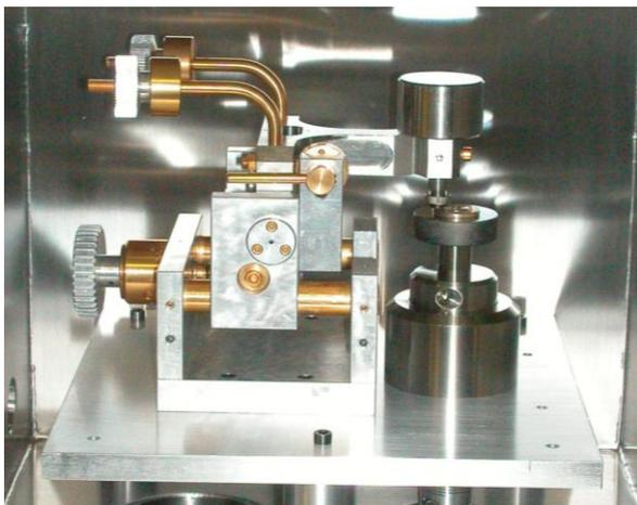
Figure 2. Pin-on-Disc (PoD) tribometer typically used for tribological assessments of SLMs
