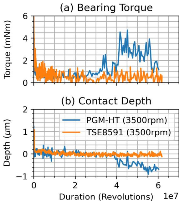
Figure 6. Comparison of (a) mean bearing torque and (b) contact depth measured in ABTR for two different SLMs
