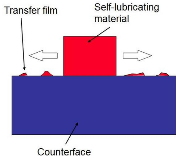
Figure 1. Sacrificial wear and transfer film production for a SLM
