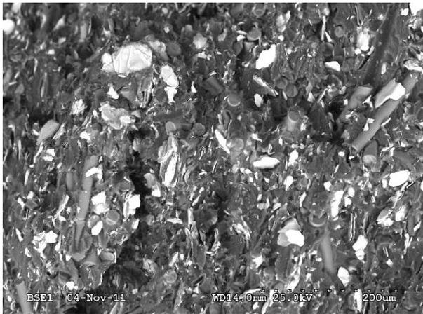
Figure 8. SEM micrograph of PGM-HT material cross-section [11]
