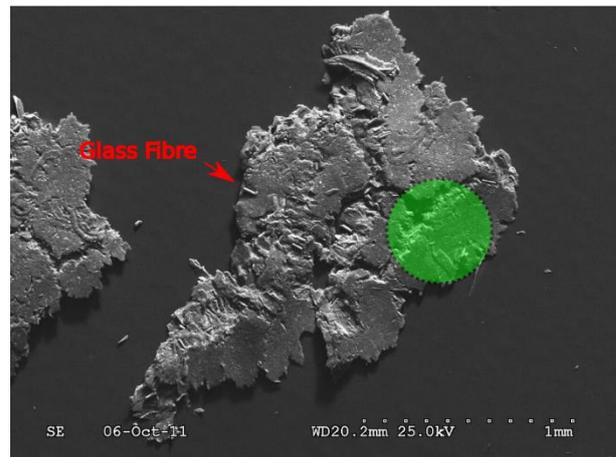
Figure 10. SEM micrograph of transferred PGM-HT material with the contact area overlaid (green circle)
