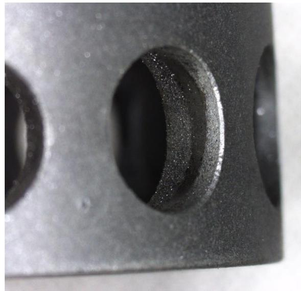
Figure 7. Post-test TSE8591 cage pocket wear
