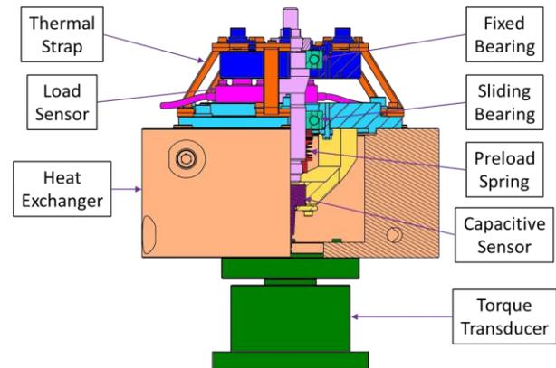
Figure 5. Internal arrangement of the ABTR
