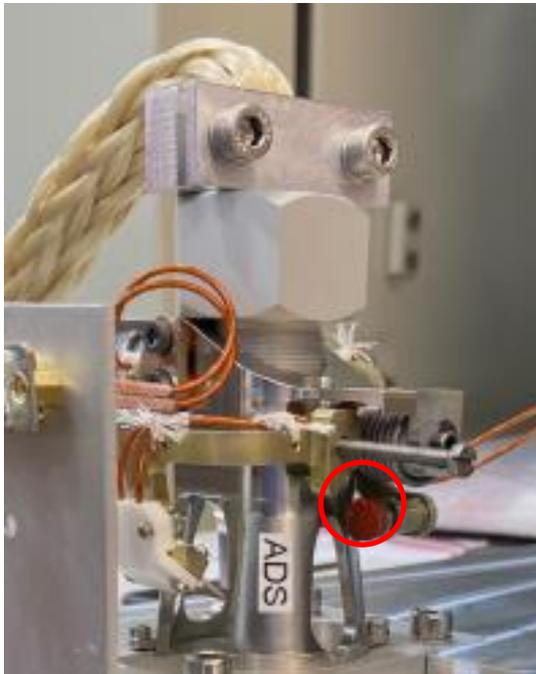
Figure 11. Stop-bolt damping.
