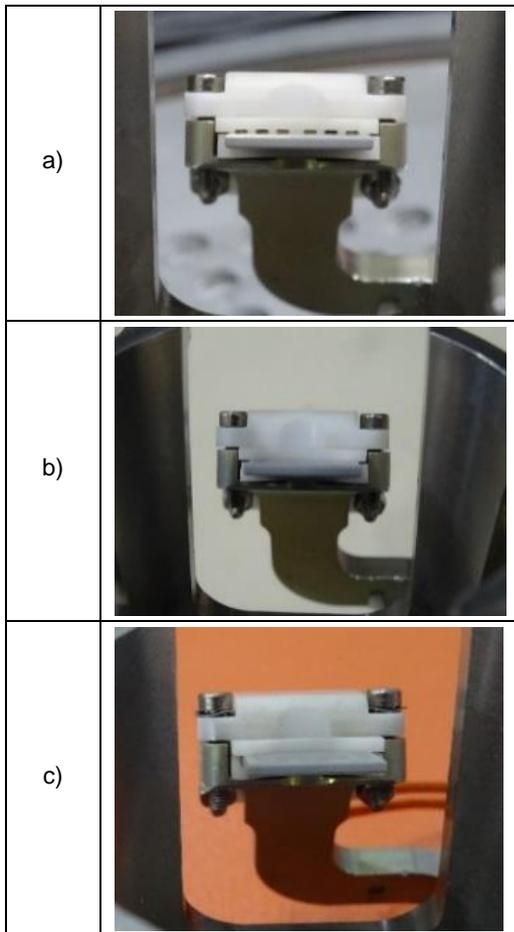
Figure 5. NELS HDRS thermal knife a) initial configuration, b) intermediate configuration with upper insulating plate without grooves and c) final configuration with upper insulating plate without grooves and crinkle washers below the screws' head.
