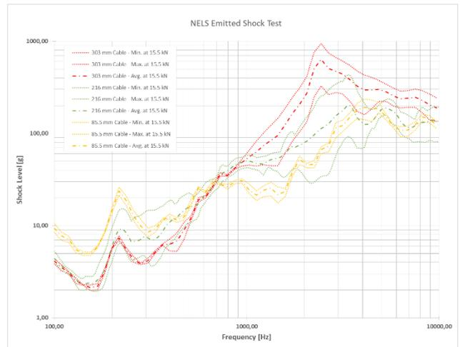
Figure 9. Emitted shock SRS measured 100mm from the axis of the NELS HDRS and relative to restraint cables with a length of 85.5 mm (yellow colour), 216 mm (green colour) and 303 mm (red colour).
