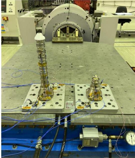
Figure 6. In-plane random vibration test setup showing QM-1 (left side) and QM-2 (right side).
