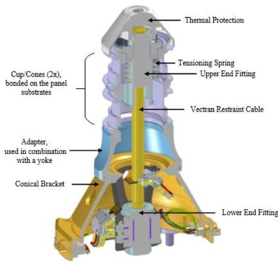
Figure 3. NELS HDRS cross-sectional view.
