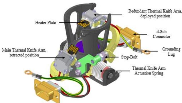
Figure 4. NELS HDRS cross-sectional view.
