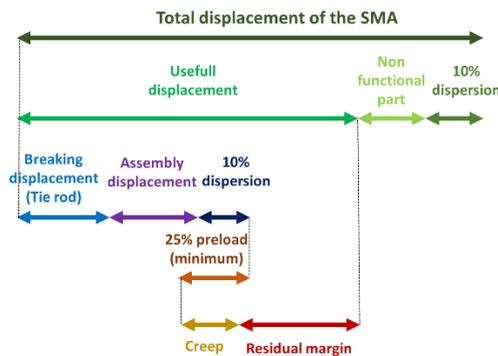
Figure 13: budget of displacement
