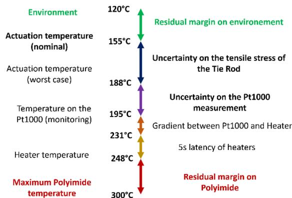
Figure 12: definition of thermal margins
