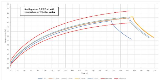
Figure 7: Heating under 0,5 W/cm<sup>2</sup> with temperature on TC1 after ageing
