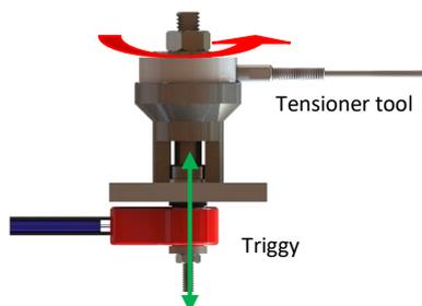
Figure 16: tensioner tool with a Triggys assembly
