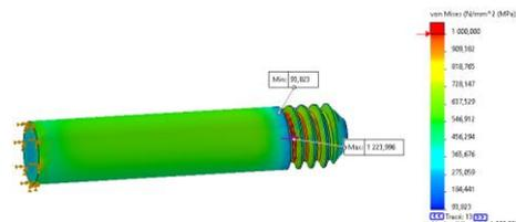
Figure 8: stress repartition on the threaded part of a Tie Rod
