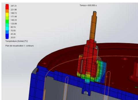
Figure 10: thermal model of Triggys at actuation
