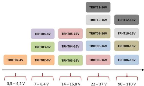
Figure 5: Available voltage for each Triggly size
