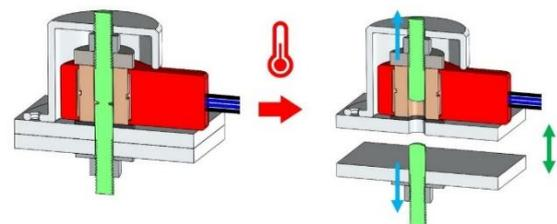
Figure 2: principle of Triggys actuation
