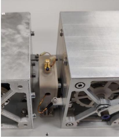
Figure 9 Balun position on the dipole antenna
