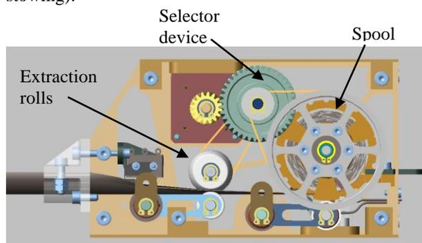
Figure 3 CTDA mechanism
