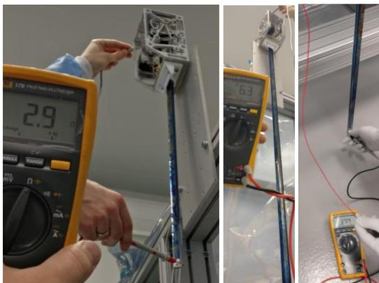
*Figure 11 Boom electrical resistance measurement*
