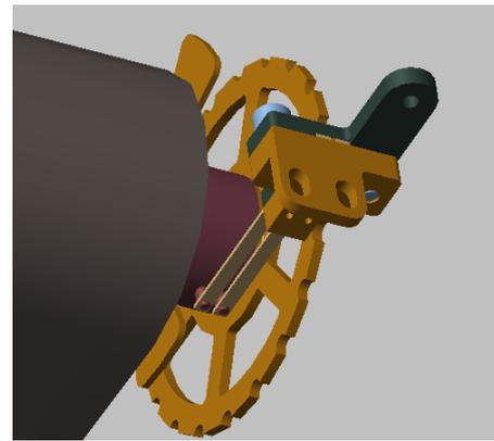
Figure 6 Electrical contact between spool and the end connection
