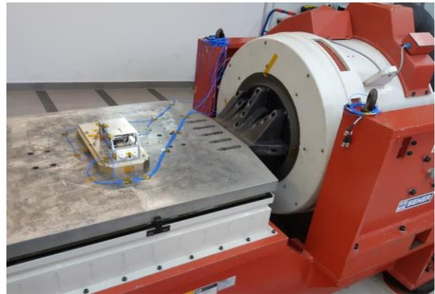
Figure 15 BBM on vibration table
