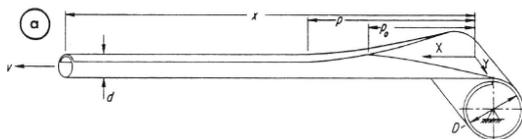
Figure 1 Deployment of single STEM
