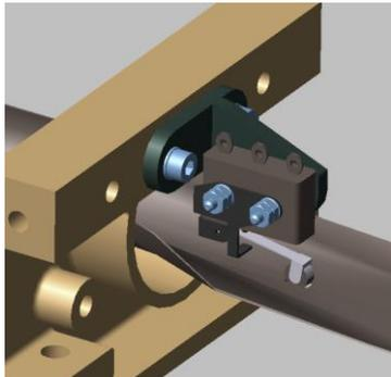
Figure 5 Length control micro switch
