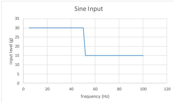
Figure 12 Sine test input (max 27g reached)
