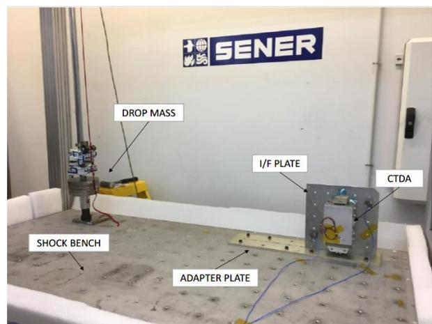
Figure 17 Shock test set-up
