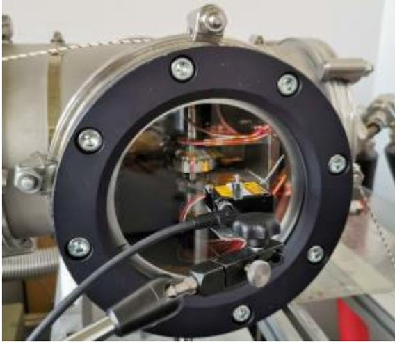
Figure 14. Lifetime setup for vacuum condition
