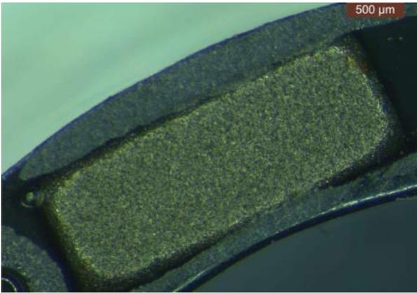
Figure 9. Uncorroded surface after humidity exposure, Sample from group B, courtesy of ESA-ESTEC
