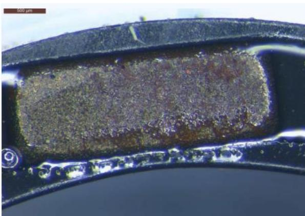
Figure 10. Surface corrosion after humidity exposure, Sample from group A, courtesy of ESA-ESTEC
