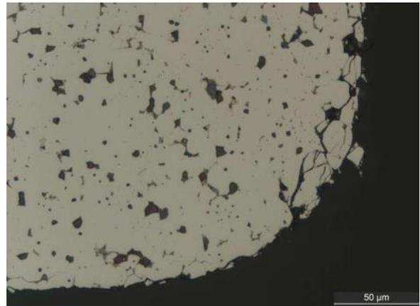
Figure 12. Micro-section of corroded sample, courtesy of ESA-ESTEC
