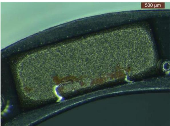
Figure 11. Surface corrosion after humidity exposure, Sample from group B, courtesy of ESA-ESTEC
