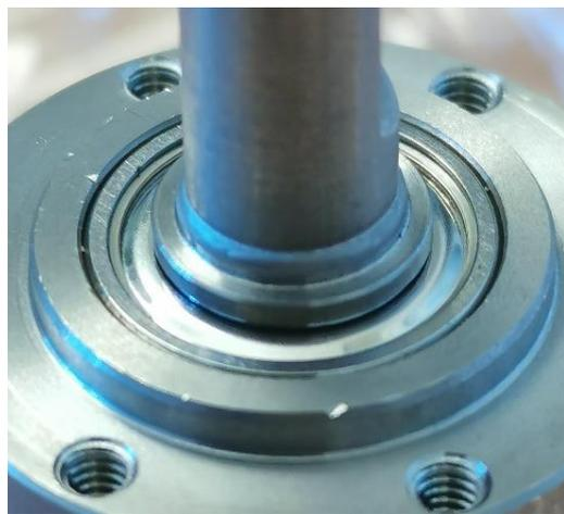
Figure 8: Laser welding spot on gearhead's output shaft
