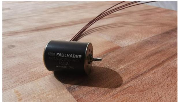
Figure 1. S2M2 Stepper Motor Series AM2224
