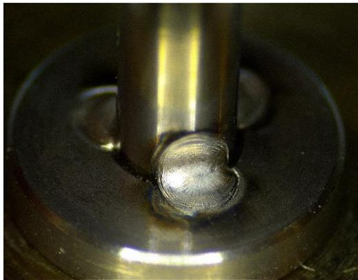
Figure 7. Laser welding spot on motor's shaft
