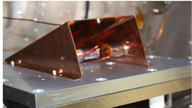
Figure 6. Test setup view (hot plate, actuator sample and baffle), courtesy of ESA-ESTEC
