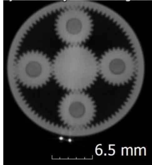
Figure 15. Tomography image of one gearhead's stage
