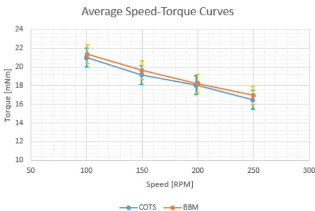
Figure 5. Average speed-torque curves for the COTS and BBM motors
