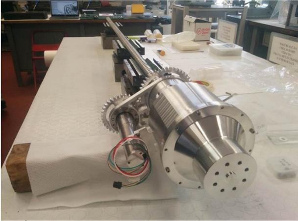
Figure 8. A drill designed to penetrate 1–2 m into the lunar surface is envisaged by ESA to fly to the Moon's south pole on Russia's Luna-27 lander in 2020. Credit: ESA/Finmeccanica.
