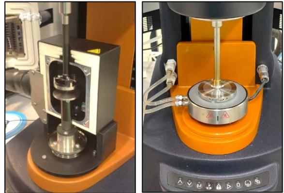
Figure 4. Left: Parallel plate inside the humidity chamber. Right: Parallel plate configuration mounted on ETC.
