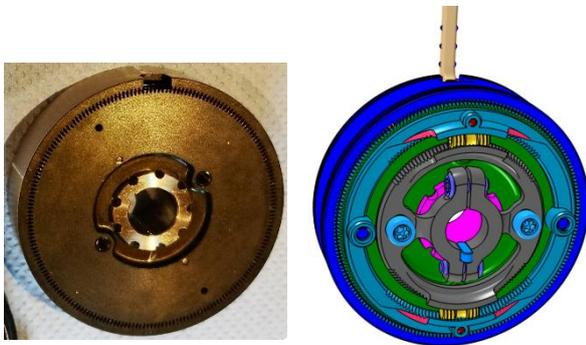
Figure 3: Breadboard model of the magnetic brake MB2R3
