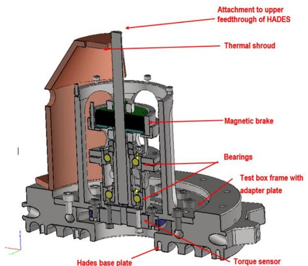
Figure 4: Breadboard TV-measurement assembly diagram
