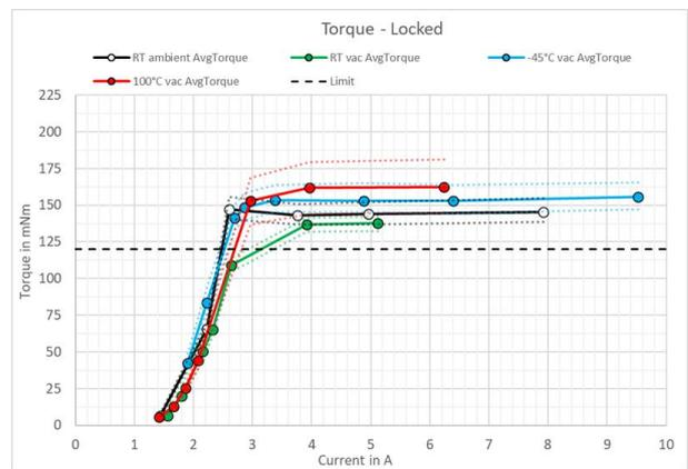
Figure 7: Measured brake performance in different environments. Plotted over the steady state current during the switching pulse.
