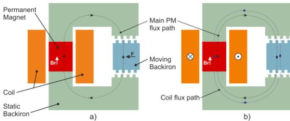
Figure 2: Simplified linear depiction of a basic reluctance magnetic circuit. a) Locked state. b) Unlocked state through active coil current.
