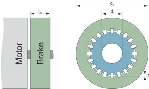
Figure 1: An example of the magnetic brake topology with 20 teeth and therefore 20 stable positions.
