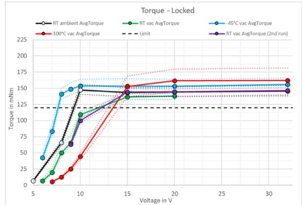
Figure 6: Measured brake performance in different environments. Above a supply voltage of 15V used for the ~100ms pulse, the brake state was fully toggled.
