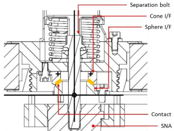
Figure 4. Sphere-cone contact interface
