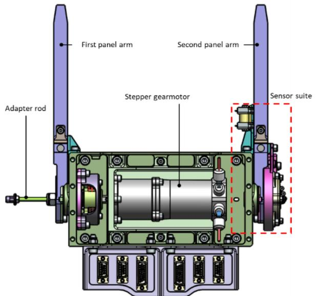
Figure 5. Actuation system top view
