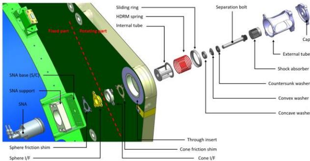
Figure 3. HDRM exploded view
