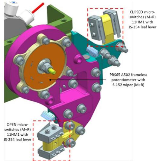
Figure 6. Actuation system sensor suite
