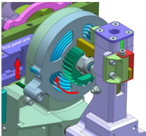
Figure 8. Emergency spring torque application
