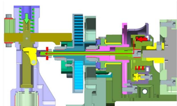
Figure 9. Initial configuration during emergency opening. The solid arrow indicates the load path
