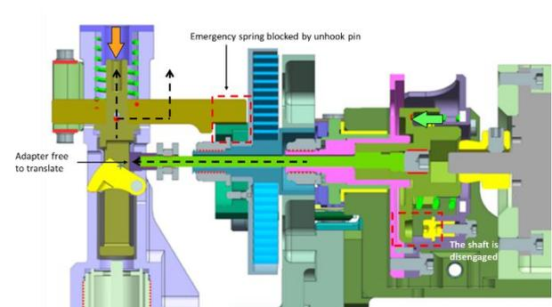
Figure 10. Gearmotor shaft decoupling. The dashed arrows indicate the direction of movement of the parts
