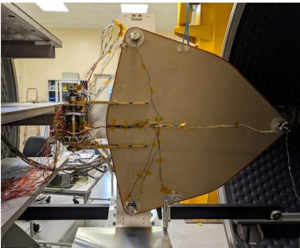
Figure 12. CDAM-CM before TVAC testing
