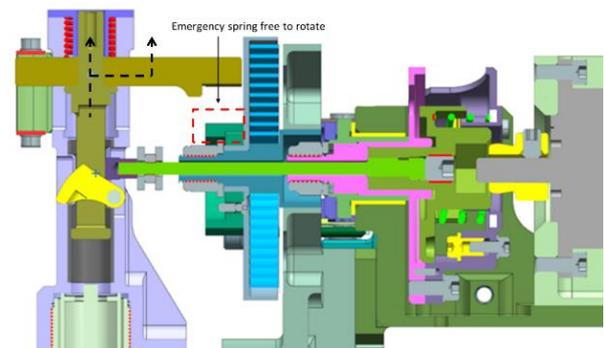
Figure 11. Emergency spring engaging. The dashed arrows indicate the direction of movement of the parts
