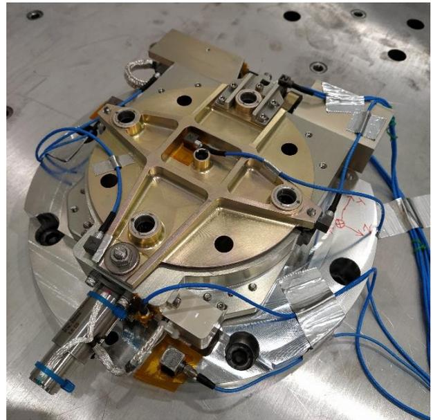
Figure 7: FDA QM during vibration test
