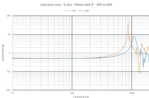
Figure 6: Motor IF resonances before and after the redesign
