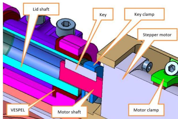
Figure 5: Cross-section of the torque transfer design
