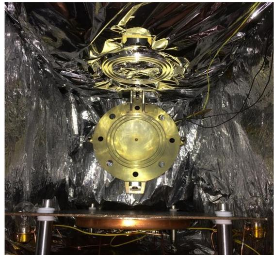
Figure 9: TVAC FDA Lid down configuration
