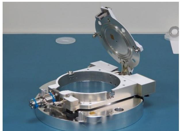
Figure 2: Partially opened FDA FM on a vibration jig
