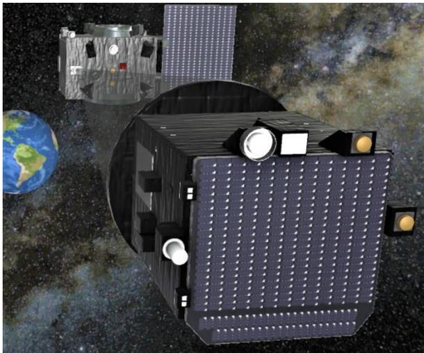
Figure 1: Proba-3 illustration - CSC (further) with FDA at the tip of the shadow cone cast by the OSC (closer)
