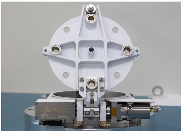
Figure 4: FDA FM – partially opened Lid and the Connector bed, the Hinge, and the Motor bed below (left to right)
