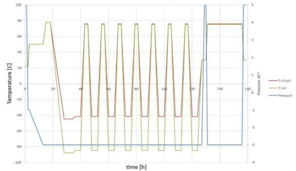
Figure 8: TVAC temperature and pressure profile
