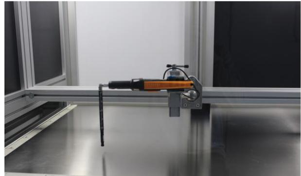
Figure 9: Flow Characterization using a hot-wire anemometer.
