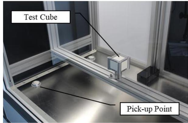
Figure 12: Test Cube and Pick-Up points
