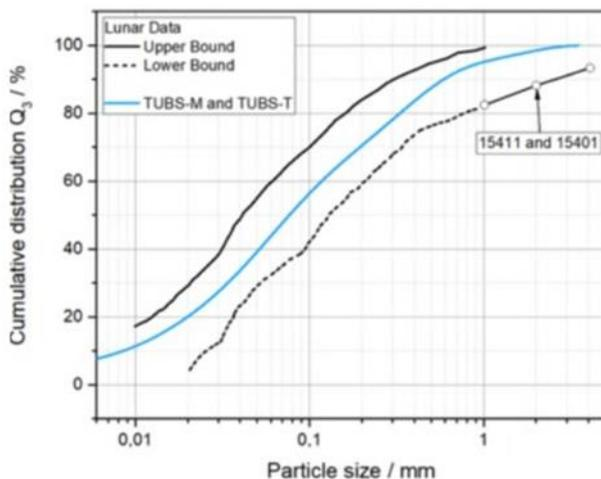
Figure 8: TUBS-M & TUBS-T Regolith Simulant Cumulative Distribution Characteristics [6]
