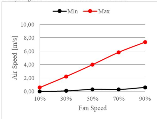
Figure 11: Minimum and maximum air speeds for different fan speed settings
