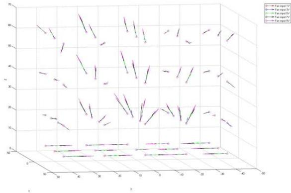
Figure 10: Stacked representation of all measured flow vectors. Vector length proportional to air speed.
