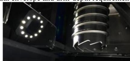
Figure 5: Drill Shell Cutting Edge Geometry
