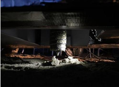
Figure 6: iDRILL testing in wet sand.
