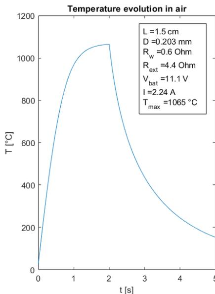
Figure 6. Nichrome wire temperature evolution in air.
