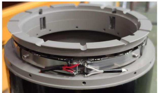
Figure 4. Redundant burn wire release system assembled on the uncoupled mechanism.
