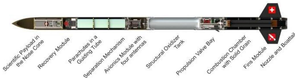
Figure 1. Longitudinal cut of the Bella Lui II rocket.
