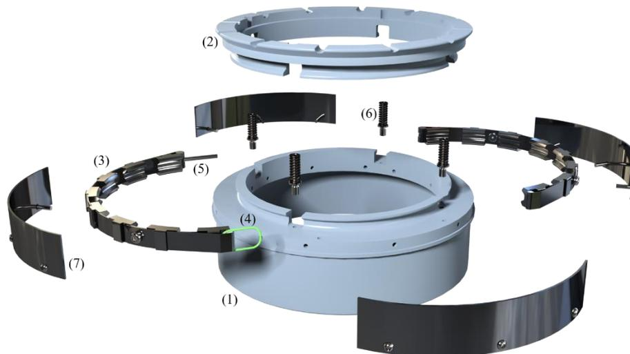
Figure 2. Exploded CAD render of the separation mechanism. (1) Lower ring, (2) Upper ring, (3) Clamp band half, (4) Dyneema loop of the burn wire release system, (5) Tensioning bolt, (6) Compression spring and guide, (7) Aero-cover.
