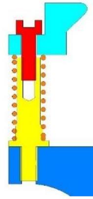
Figure 5. Temporary assembly bolt maintaining the spring compressed and rings aligned during assembly.
